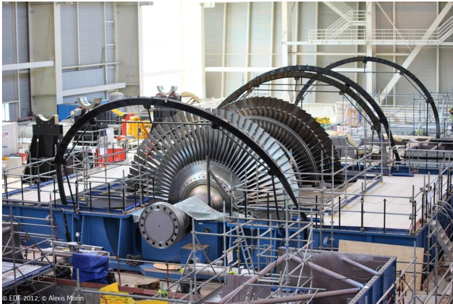
Arabelle™ steam turbine (General Electric, from 700 to 1900 MWe)
