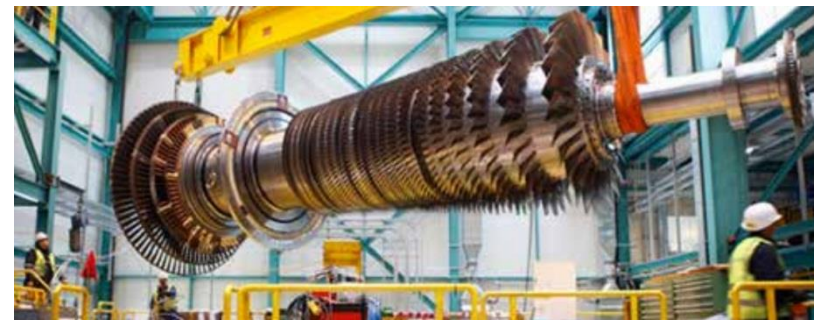
GT26 gas turbine (General Electric, 345 MWe)
